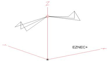
The two up-turned ends fitted nicely into the available space and provide additional end loading.
