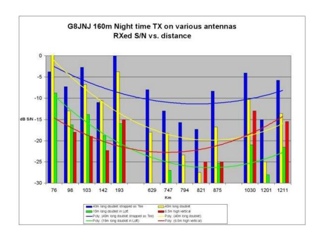
However from the WSPR results it can be seen that it actually has about 8dB less gain than the doublet, or 6dB worse than the modelled value. This loss is also consistent with measurements I made on 80m and the HF bands, and as I'm using the same ATU for both antennas, I've concluded that the loft antenna suffers as a result of coupling a fair proportion of radiated energy into mains wiring, pipe work and other structural components.
