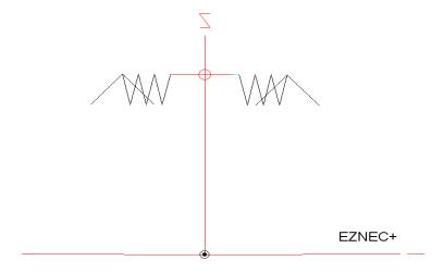
This lowered the resonant frequency which improved the performance on 80m slightly; however it still proved a difficult match on some of the HF bands, where it was approaching ½ wave long.
