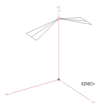
This looked promising, but then I remembered that I'd seen end loaded versions of these and also Biconical antennas being used for EMC testing. I knew they could offer a wide operating bandwidth, but that they had a 200 Ohm feed impedance, however this would be relatively easy to match via a 4:1 balun.
