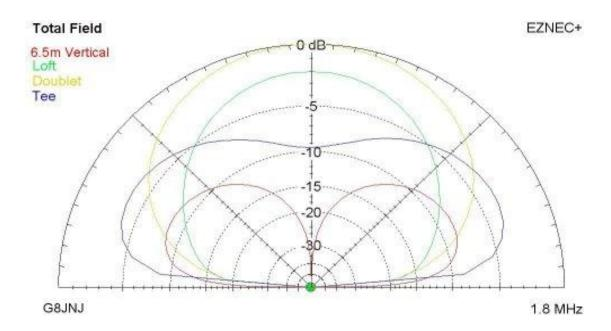
EZNEC plots I have produced for the four antennas used in the tests.
